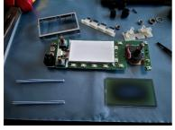
Now we can get to work on the screen. Start by removing the film on the display as shown below.
